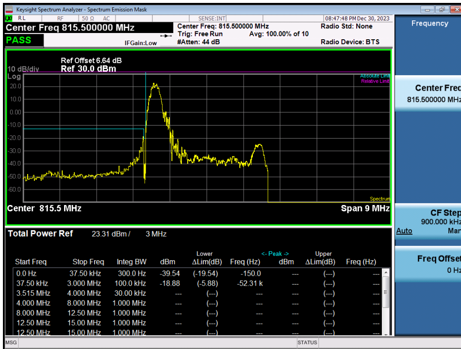
LTE Band 26 / 3 MHz / 16QAM - RB Size/Offset (1/0)
