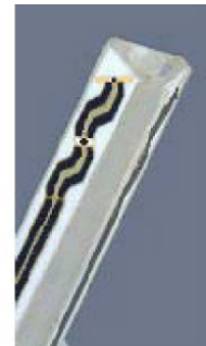
Figure 3.3 Probe Thick-Film Technique
