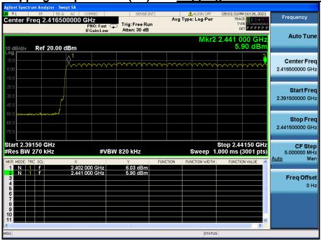
Number of Hopping Frequencies 2(FH) <u>Hopping mode : Enable & 8DPSK</u>
