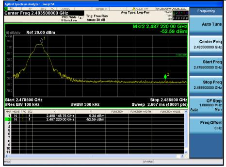
High Band-edge <u>Hopping mode & Modulation : GFSK</u>
