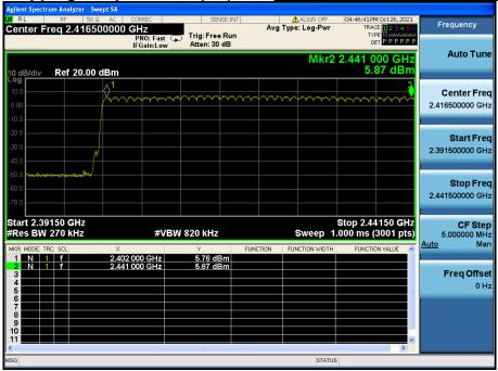
Number of Hopping Frequencies 2(FH) <u>Hopping mode : Enable & π/4DQPSK</u>
