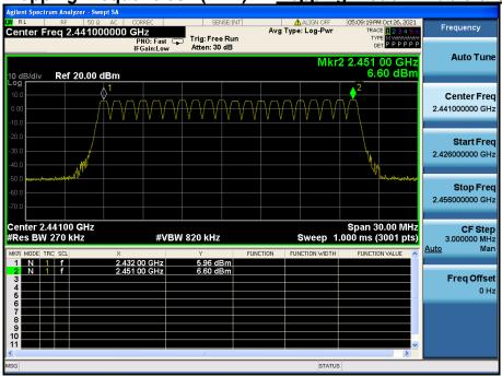
Number of Hopping Frequencies 1(AFH) <u>Hopping mode : Enable & π/4DQPSK</u>
