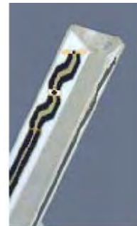
Figure E.2.2 Probe Thick-Film Technique
