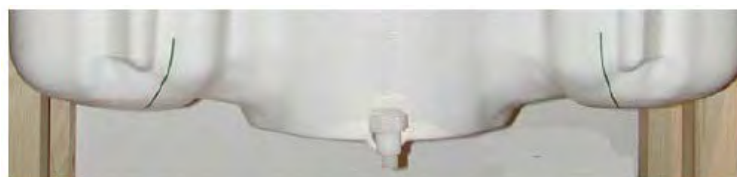
Figure 3.7 Sam Twin Phantom shell
