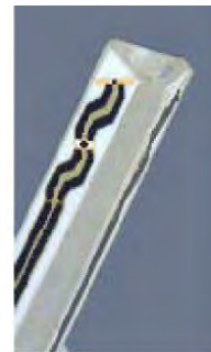
Figure 3.3 Probe Thick-Film Technique
