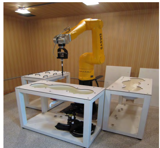
Figure 4.1 DASY5 Test System
