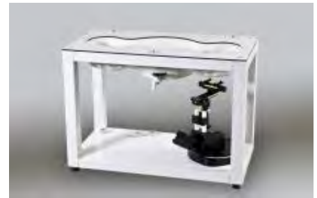
Figure 3.6 SAM Twin Phantom
