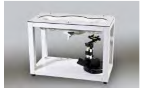
Figure E.5.1 SAM Twin Phantom
