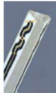
Figure E.2.2 Probe Thick-Film Technique
