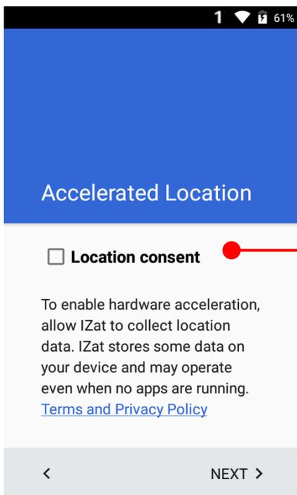
PM550's default setting is **High accuracy** mode which use GPS, WLAN for accurate location tracking. If you want to enable hardware acceleration as well, please check **Location consent**
