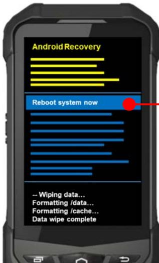
After data wiping, please select "Reboot system now" to finish the "Force Factory data reset" process
