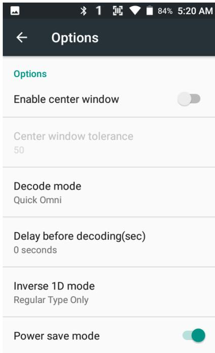
In the “Options”, you can enable/disable the “Center Window”, set “Decode mode”, “Power save mode” and enable/disable “Aimer” & “Illumination” option
