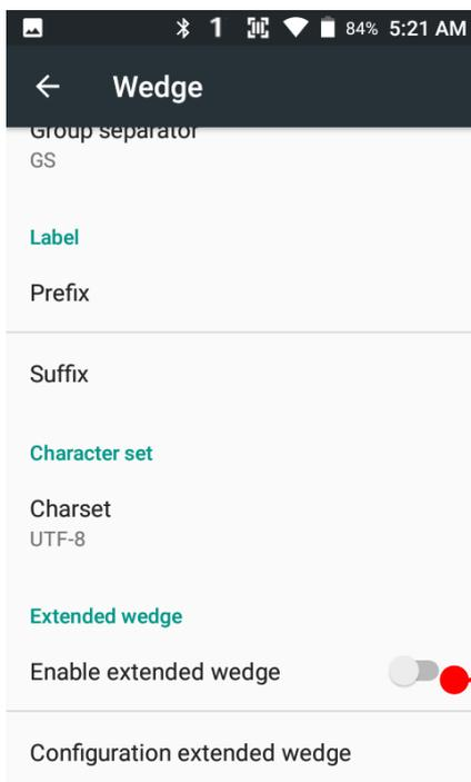
PM550 has decoded data edit function. You can add or remove specific data from decode value. To use this function, enable the option and then set a rule
