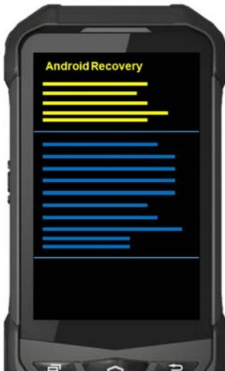
PM550 enter to the “Android Recovery” mode. In this mode, all key pad pressing move down the menu tree and “Power Button” is “Select”
