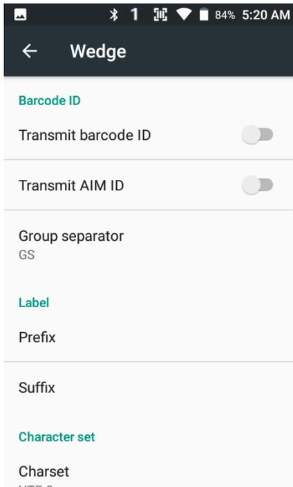
In the “Wedge”, you can enable/disable “Barcode ID” and “AIM ID”, set “Group separator”, “Prefix” & “Suffix”, “Character set” and “Extended Wedge”
