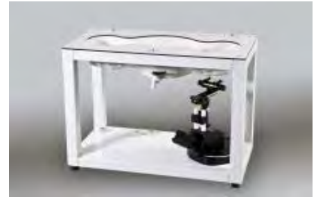
Figure E.5.1 SAM Twin Phantom
