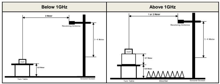
These measurements were performed at 3 m test site. The equipment under test is placed on a non-conductive table 0.8 meter or 1.5 meter above a turntable which is flush with the ground plane and 3 meters from the receive antenna. For measurements above 1GHz absorbers are placed on the floor between the turn table and the antenna mast in such a way so as to maximize the reduction of reflections. For measurements below 1 GHz, the absorbers are removed.
