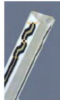
Figure E.2.2 Probe Thick-Film Technique
