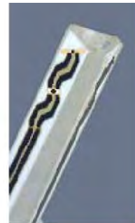
Figure E.2.2 Probe Thick-Film Technique
