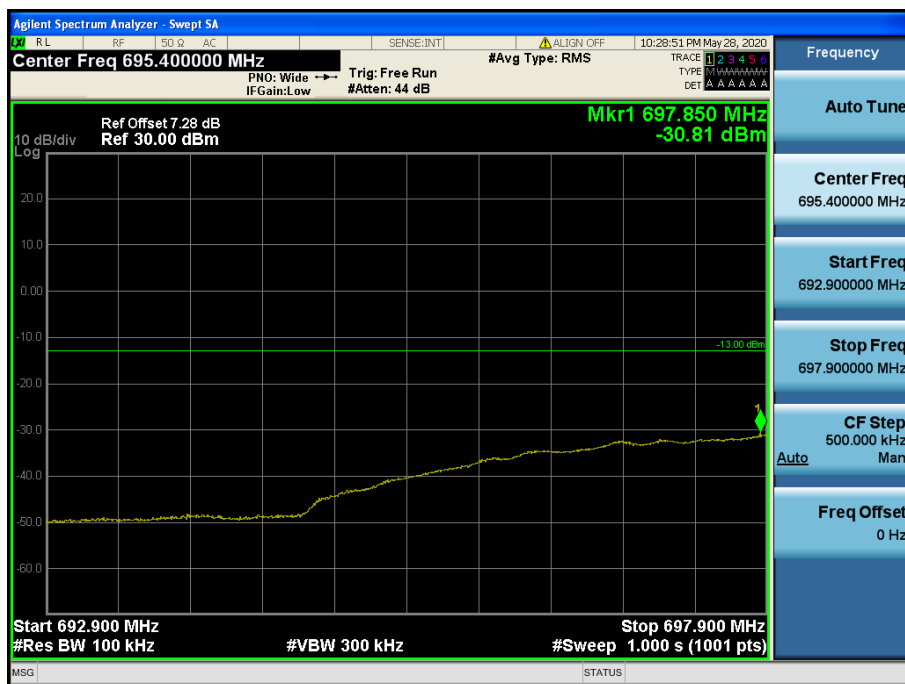
LTE Band 12, 17 / 5 MHz / QPSK RB - Size/Offset (25/0)
