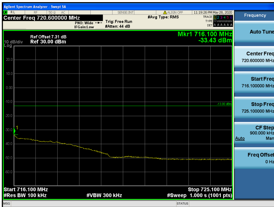
LTE Band 12, 17 / 10 MHz / QPSK - RB Size/Offset (25/25)
