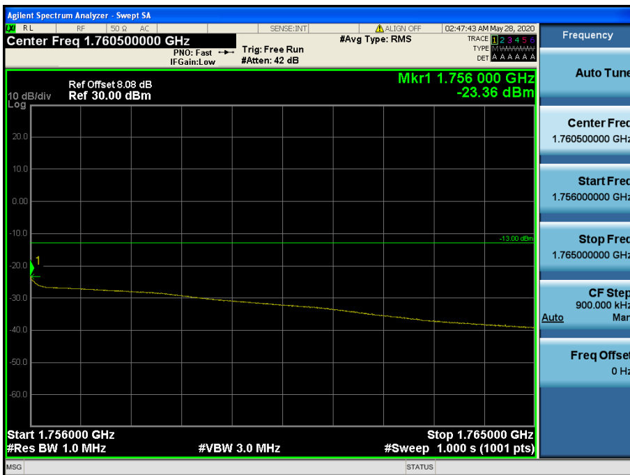
LTE Band 4 / 10 MHz / 16QAM - RB Size/Offset (25/25)
