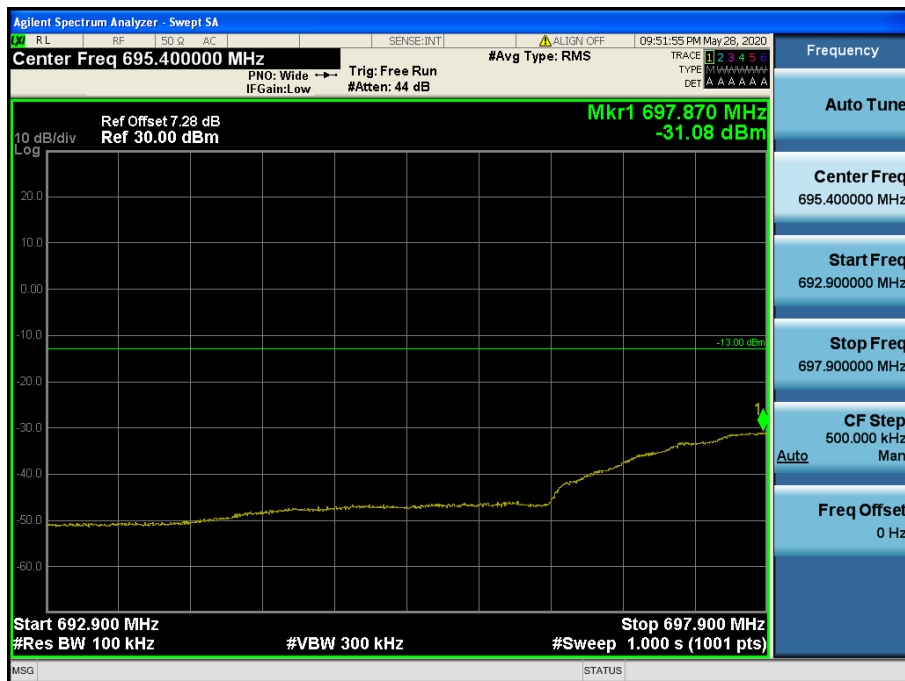
LTE Band 12 / 3 MHz / QPSK - RB Size/Offset (15/0)
