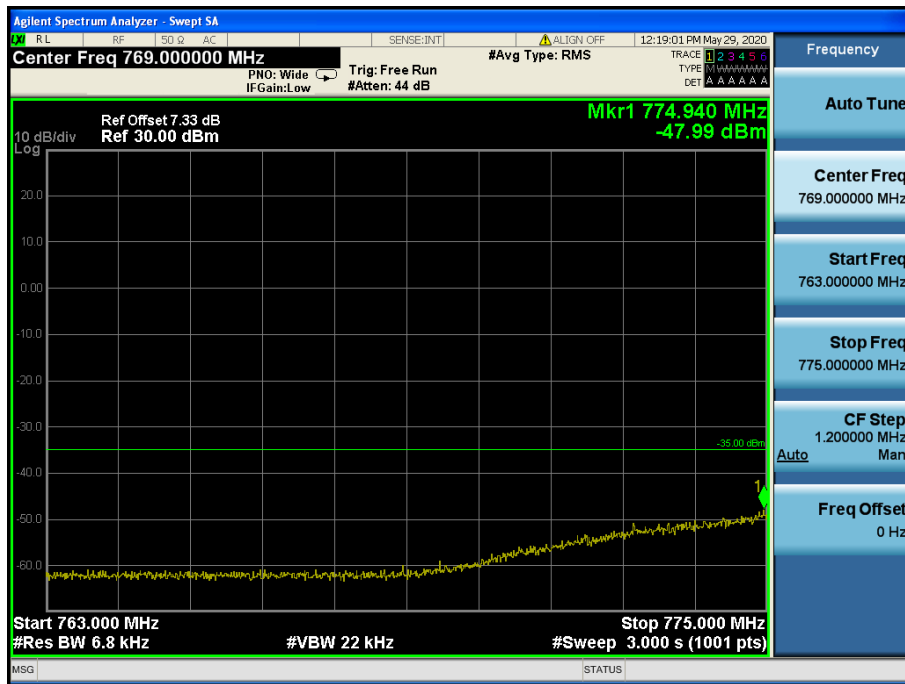
LTE Band 13 / 10 MHz / 16QAM - RB Size/Offset (50/0)
