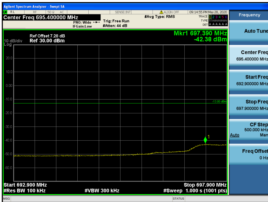
LTE Band 12 / 1.4 MHz / QPSK - RB Size/Offset (6/0)
