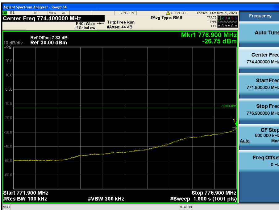
LTE Band 13 / 5 MHz / QPSK - RB Size/Offset (12/0)
