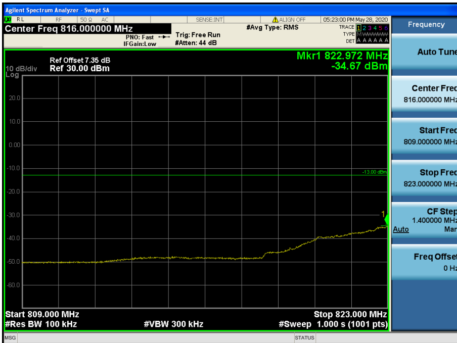
LTE Band 26 / 15 MHz / QPSK - RB Size/Offset (36/0)
