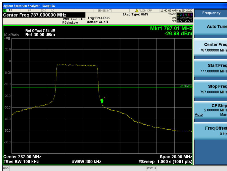
LTE Band 13 / 10 MHz / QPSK - RB Size/Offset (25/25)
