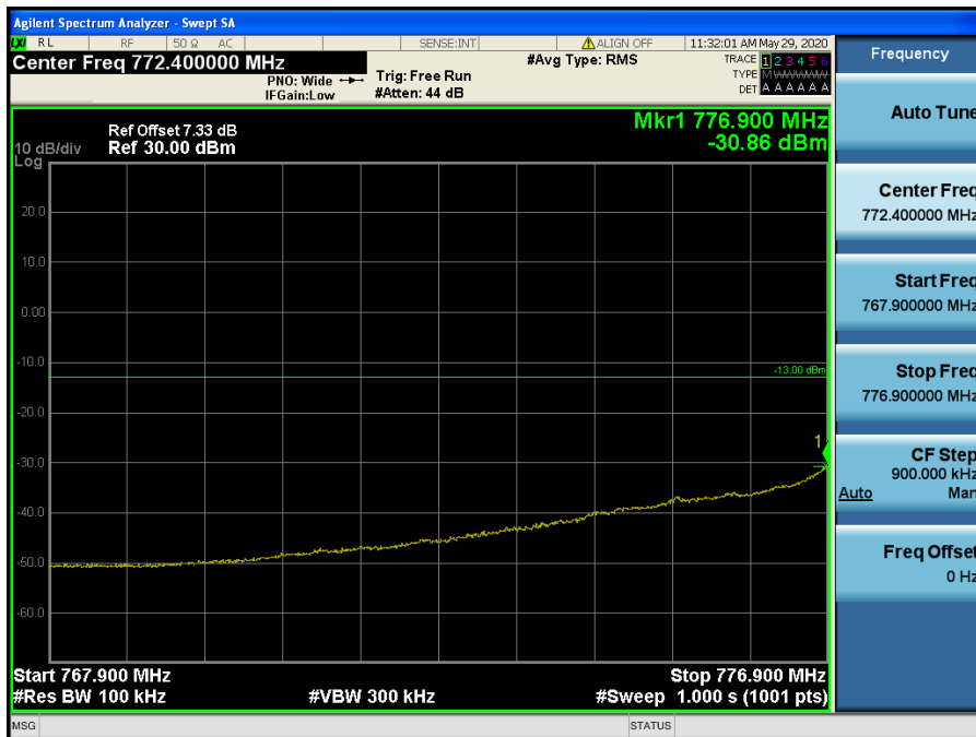
LTE Band 13 / 10 MHz / QPSK - RB Size/Offset (25/0)
