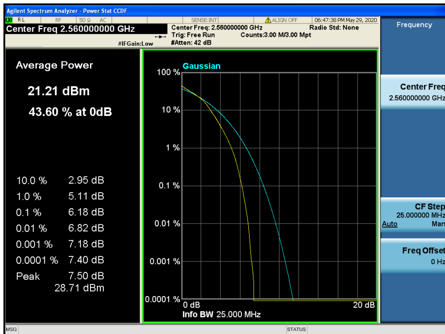
LTE Band 7 / 20 MHz / 16QAM - RB Size 100
