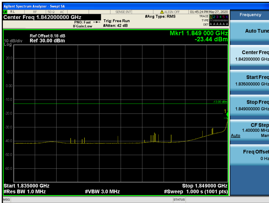
LTE Band 2 / 15 MHz / QPSK - RB Size/Offset (1/0)
