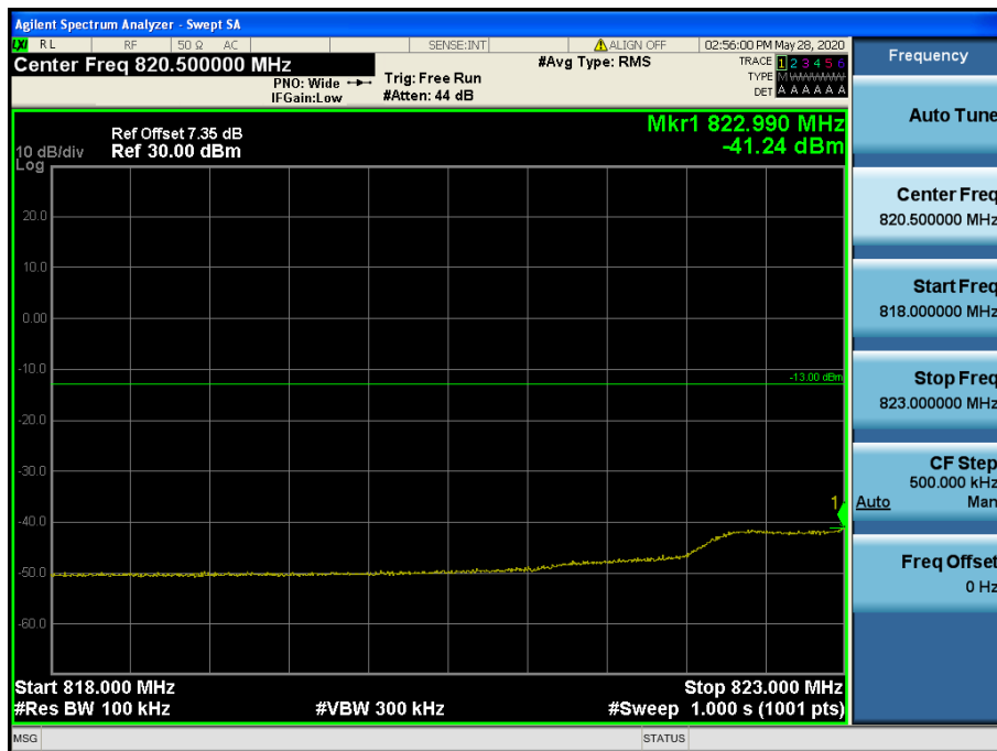
LTE Band 26 / 1.4 MHz / QPSK - RB Size/Offset (6/0)
