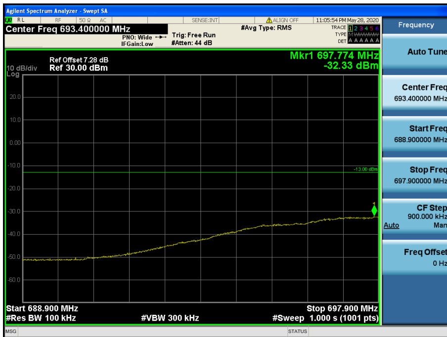
LTE Band 12, 17 / 10 MHz / QPSK - RB Size/Offset (50/0)
