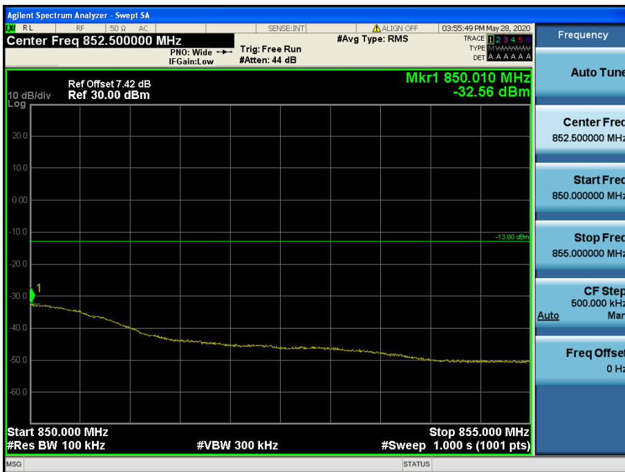
LTE Band 26 / 3 MHz / QPSK - RB Size/Offset (15/0)
