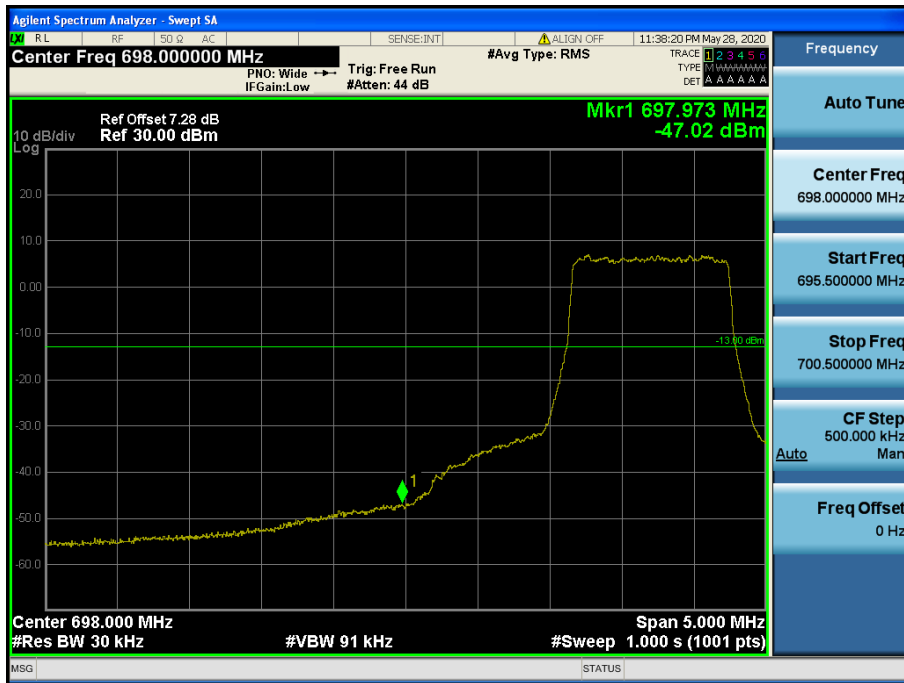
LTE Band 12 / 1.4 MHz / 16QAM - RB Size/Offset (6/0)
