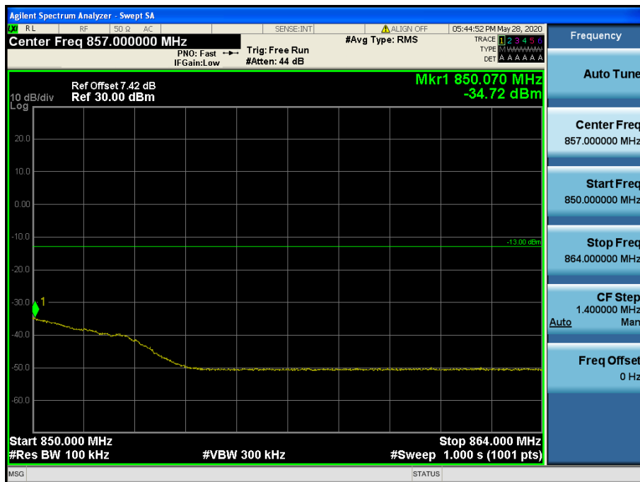
LTE Band 26 / 15 MHz / QPSK - RB Size/Offset (36/39)
