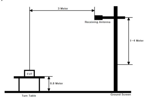
These measurements were performed at 3&10m test site. The equipment under test is placed on a non-conductive table 0.8-meters above the ground plane and 3-meters from the receive antenna.
