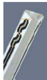
Figure 3.3 Probe Thick-Film Technique
