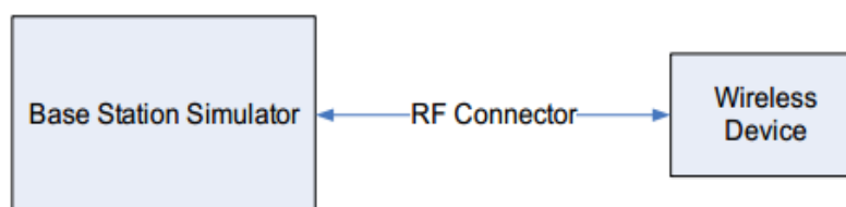
Figure 10.2 Power Measurement Setup
