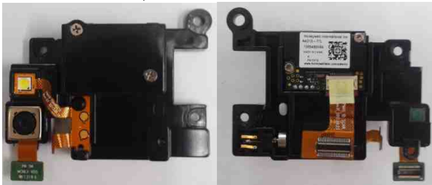
12. Scanner Bracket Module Ass'y-1 (PM40G152146K0C/PM40G152246K0C)
