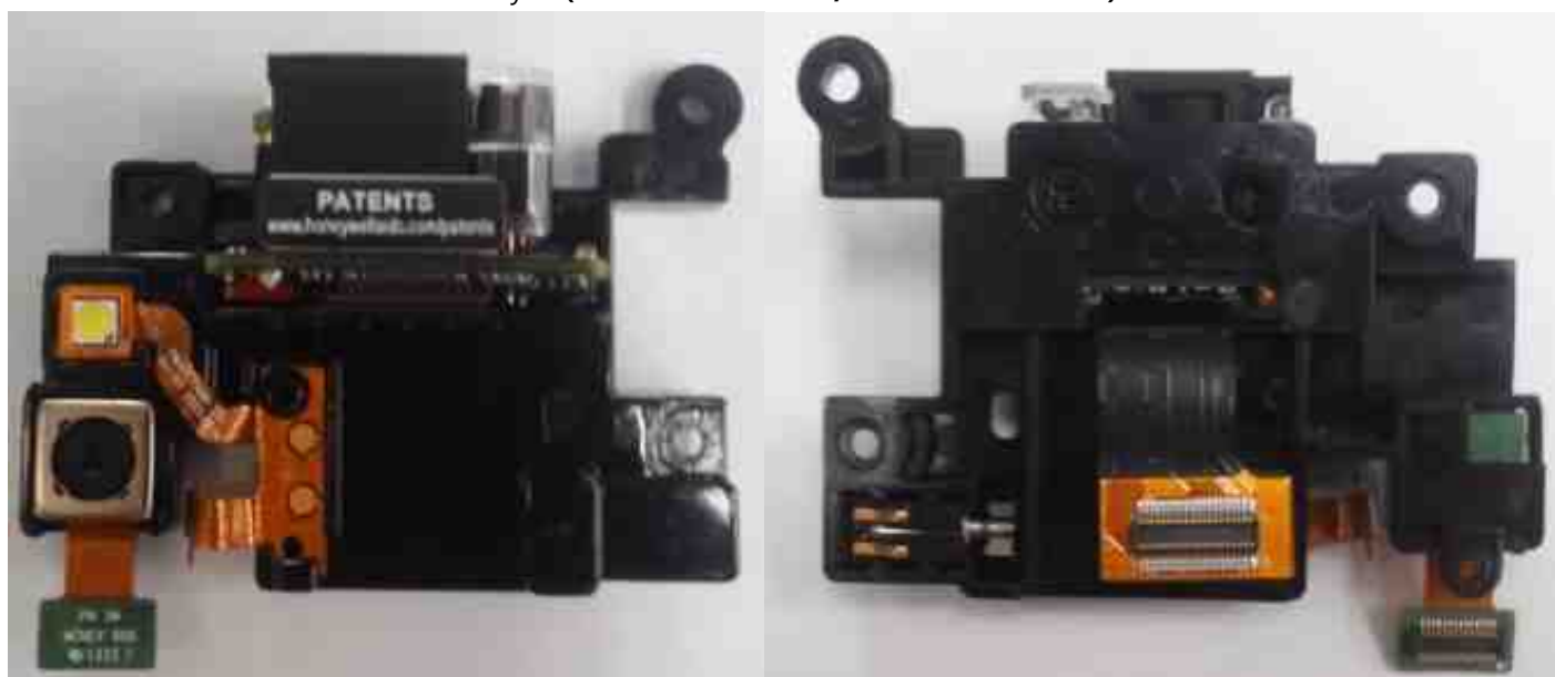
13. Scanner Bracket Module Ass'y-2 (PM40G172146K0C/PM40G172246K0C)
