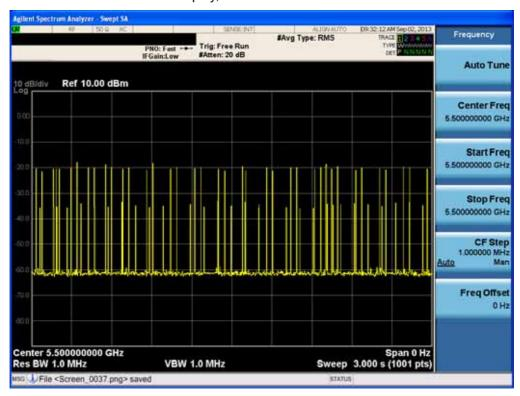
Time Display, WLAN Channel Traffic (Streaming Video)
