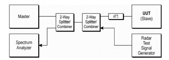
Figure 3-1. Conducted Test Setup for DFS
