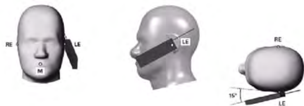
Figure 4.3 Front, Side and Top View of Ear/15° Position
