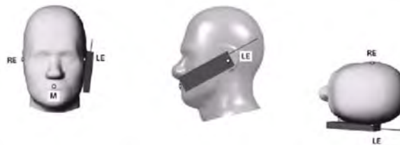
Figure 4.1 Front, Side and Top View of Cheek/Touch Position
