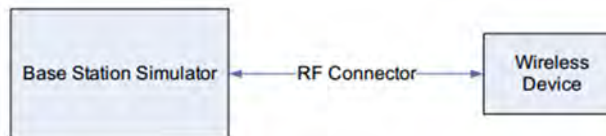
Figure 9.1 Power Measurement Setup
