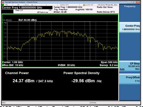
PAPR (dB) = P<sub>Pk</sub> (dBm) - P<sub>Avg</sub> (dBm) = 27.34 dBm - 24.37 dBm = 2.97 dB
