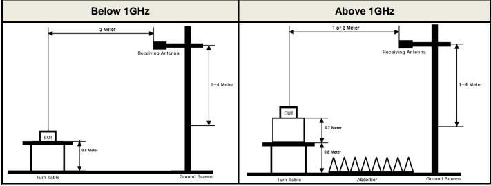
These measurements were performed at 3 m test site. The equipment under test is placed on a non-conductive table 0.8 or 1.5 meters above a turntable which is flush with the ground plane and 3 meters from the receive antenna. For measurements above 1 GHz absorbers are placed on the floor between the turn table and the antenna mast in such a way so as to maximize the reduction of reflections. For measurements below 1 GHz, the absorbers are removed.
