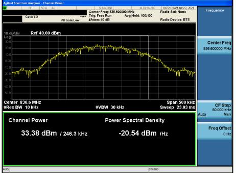
PAPR (dB) = P<sub>Pk</sub> (dBm) - P<sub>Avg</sub> (dBm) = 33.58 dBm - 33.38 dBm = 0.20 dB
