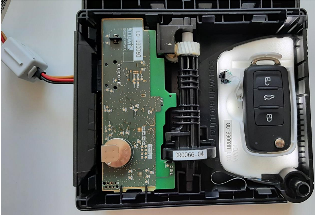
flinkey CAN lower part with keyfob and KPC (example), LEDs switched on
