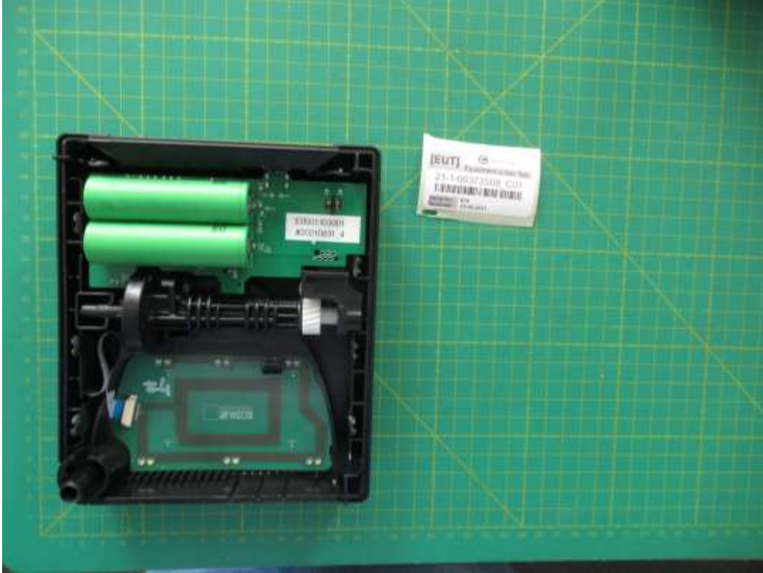
Fig. Int.: 1 : Internal view of integrated antenna
