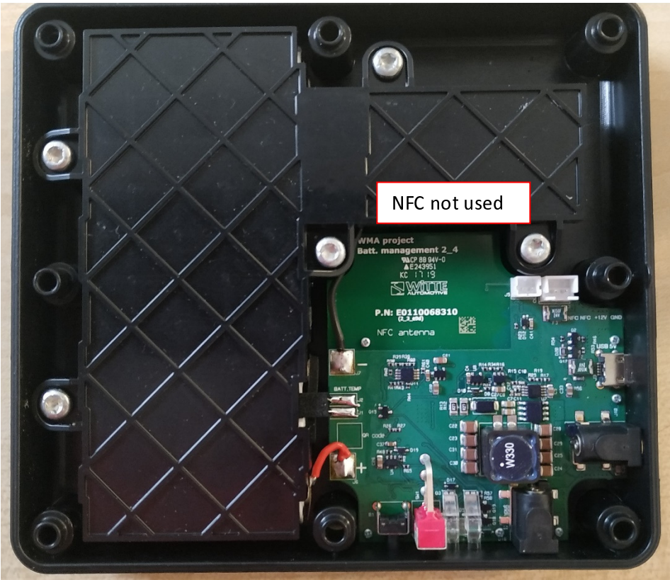
Enclosure with Battery pack and PCB 2
