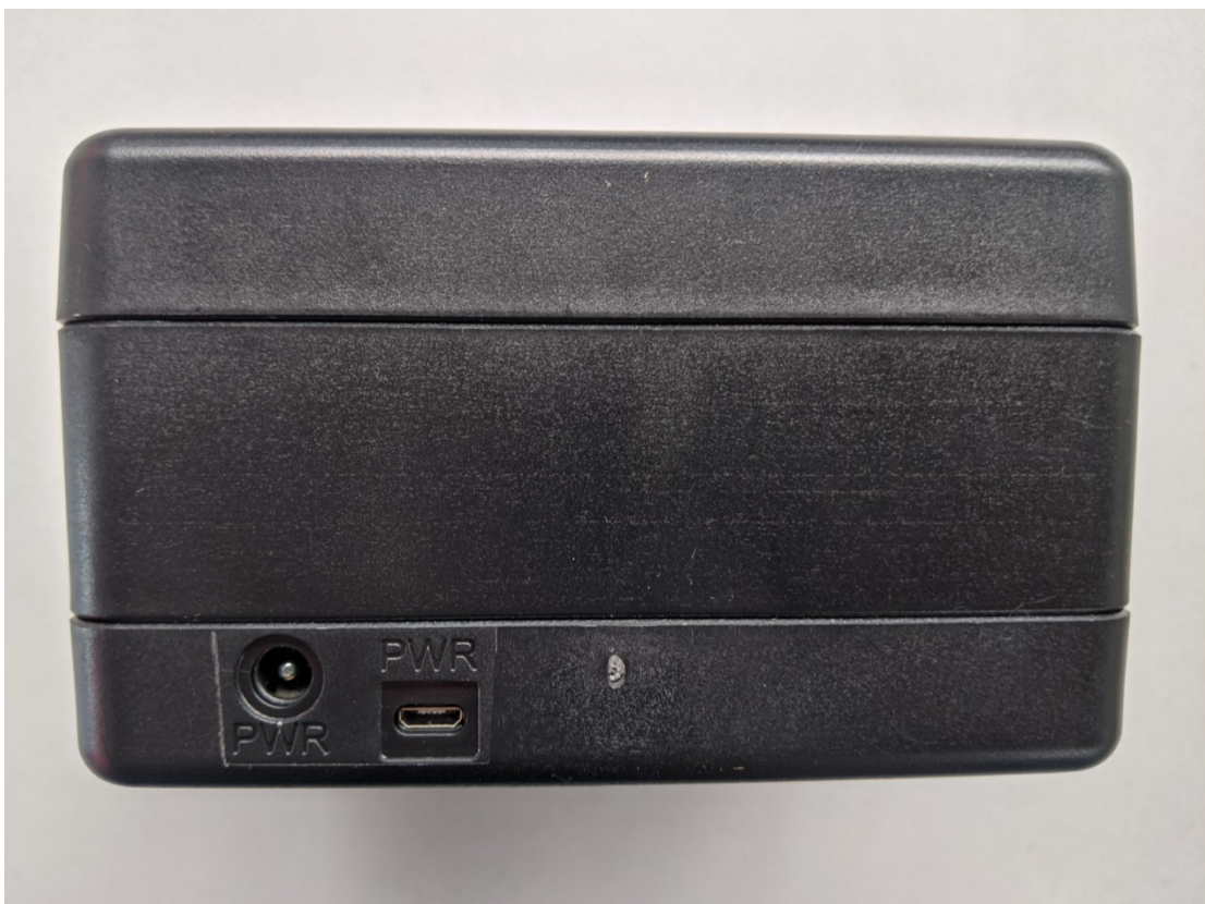
flinkey Box side view (4) with power connection for car adapter
