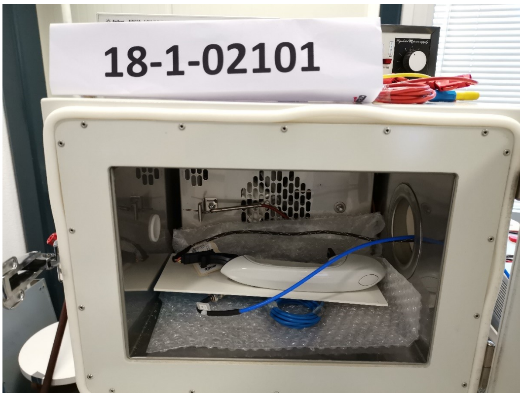
Photograph 5: close view in the radio lab. EUT in the climatic chamber.
