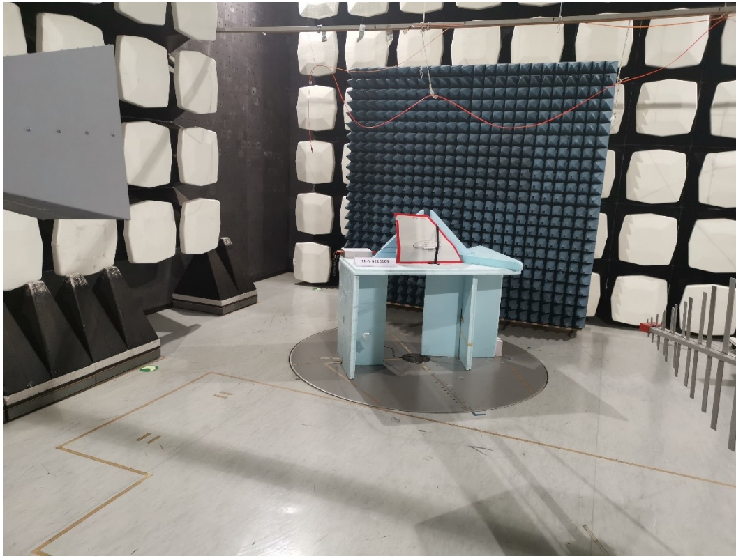
Photograph 2: overview in the semi-anechoic chamber. EUT standing.
