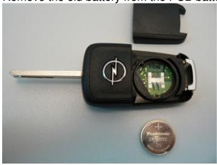
Replace the new battery with +V side facing upwards. Avoid touching the new batteries with your fingers. Skin oil may cause battery deterioration.
