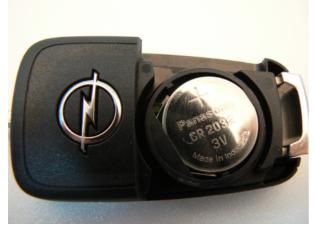
Do not touch the printed circuit board or the PCB battery holder. To reassemble the transmitter case, snap the battery box cover to the housing lower shell. Make sure that the battery box cover reliably engage.
