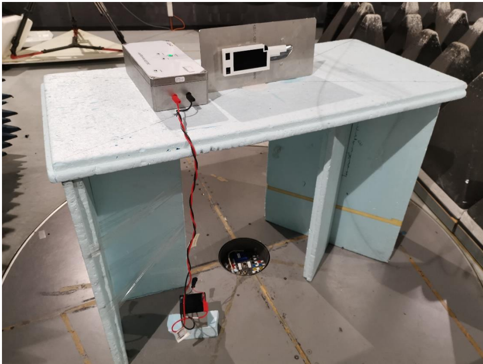
Photograph 2: Close view of the test setup in the semi-anechoic chamber. EUT stands.
