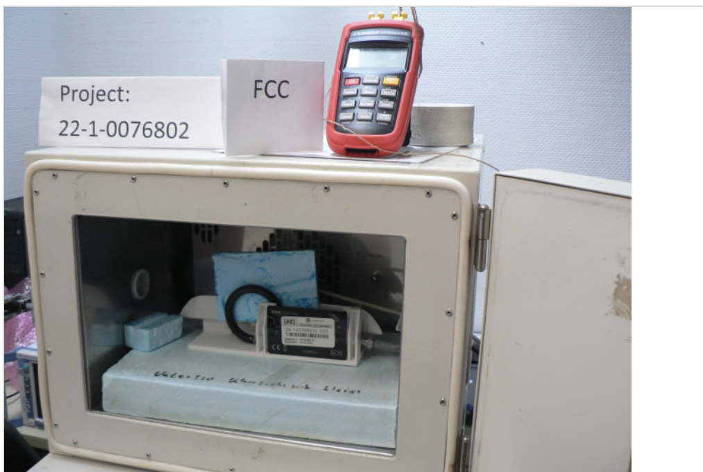
Photograph 2: Setup for extreme temperature measurement, close up view, with NFC-Tag
