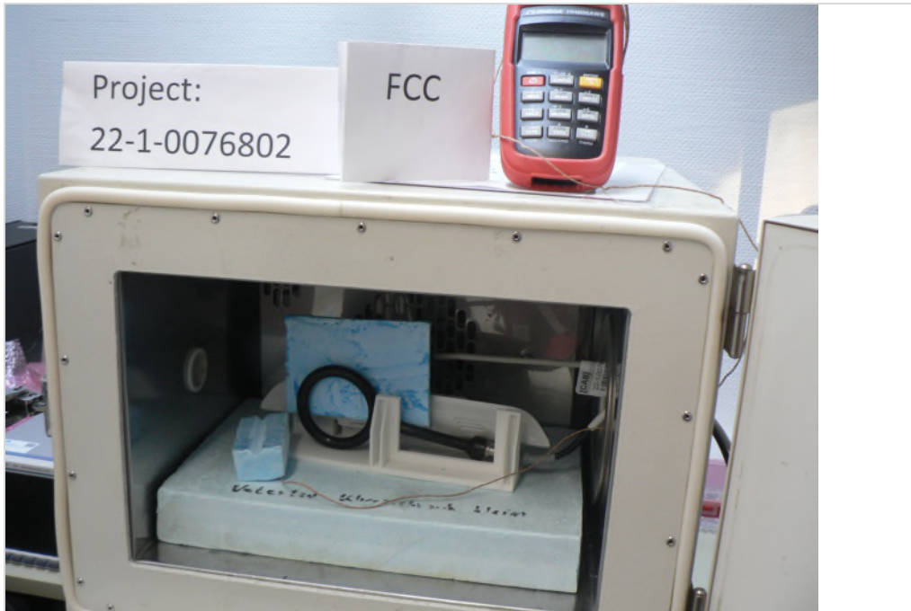
Photograph 1: Setup for extreme temperature measurement, close up view, without NFC-Tag
