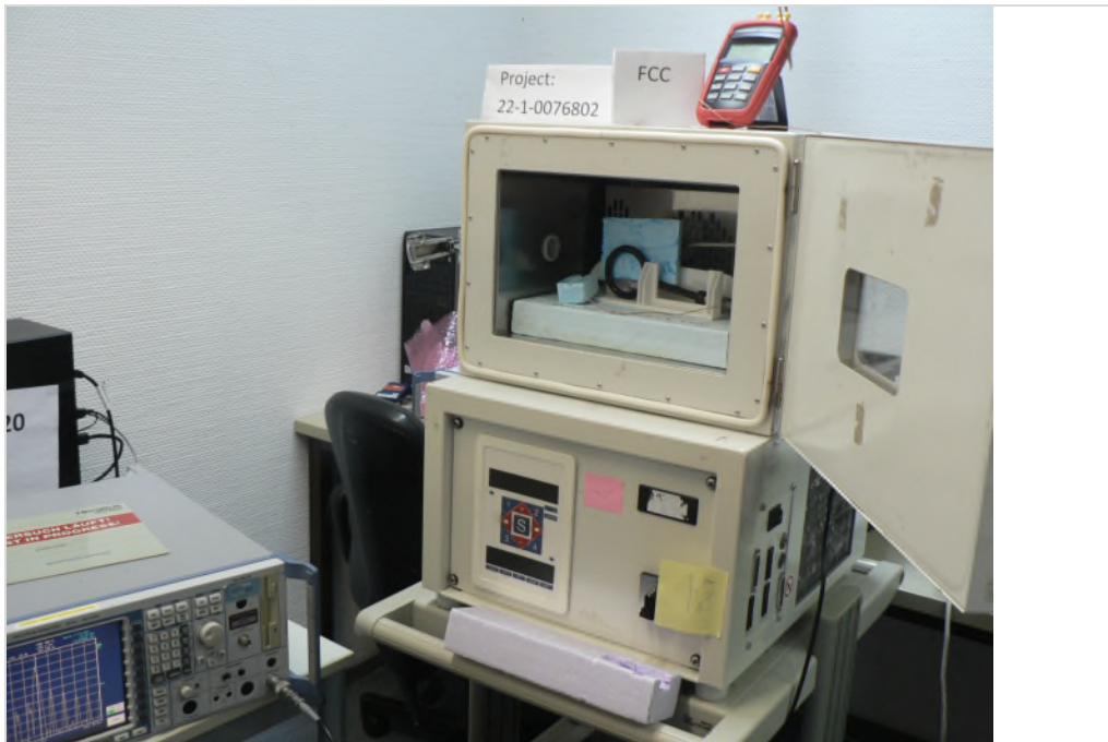
Photograph 3: Setup for extreme temperature measurement, overview
