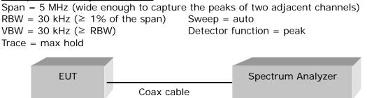
Figure 1 : Measurement setup for the carrier frequency separation
