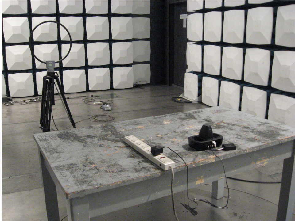
Photograph 4: Set-up for Spurious Emissions 30MHz – 1GHz
