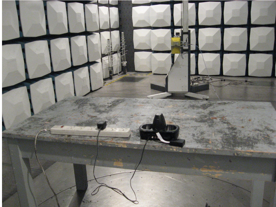
Photograph 6: Set-up for Spurious Emissions 18GHz – 26.5GHz
