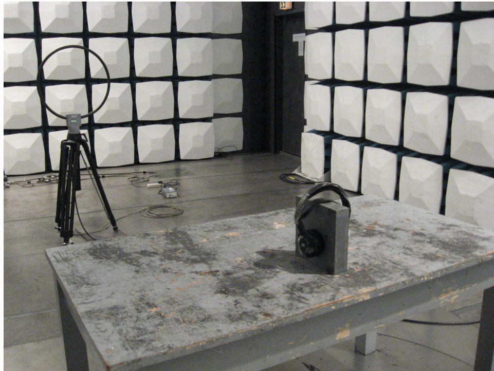
Photograph 2: Set-up for Receiver Spurious Emissions 30MHz – 1GHz
