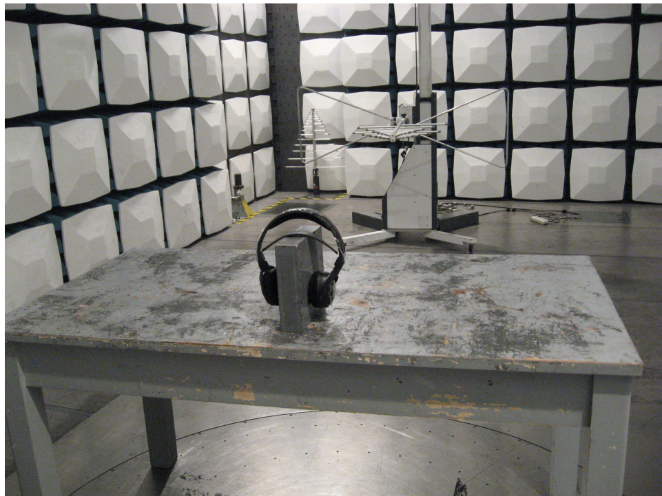
Photograph 2: Set-up for Receiver Spurious Emissions 30MHz – 1GHz
