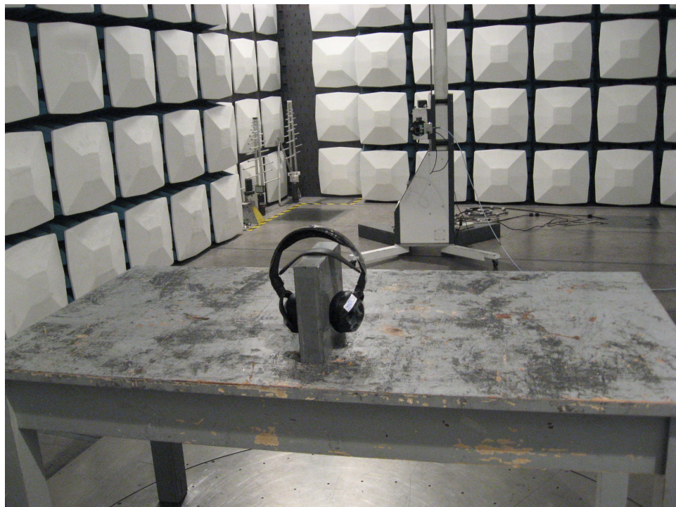
Photograph 4: Set-up for Receiver Spurious Emissions 18GHz – 26.5GHz
