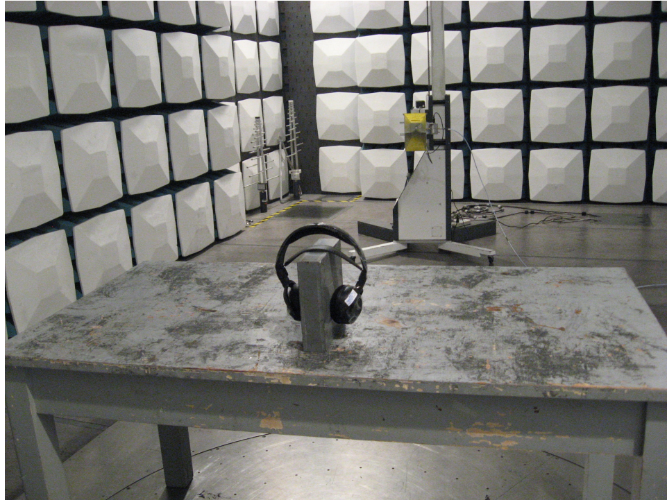
Photograph 4: Set-up for Receiver Spurious Emissions 18GHz – 26.5GHz
