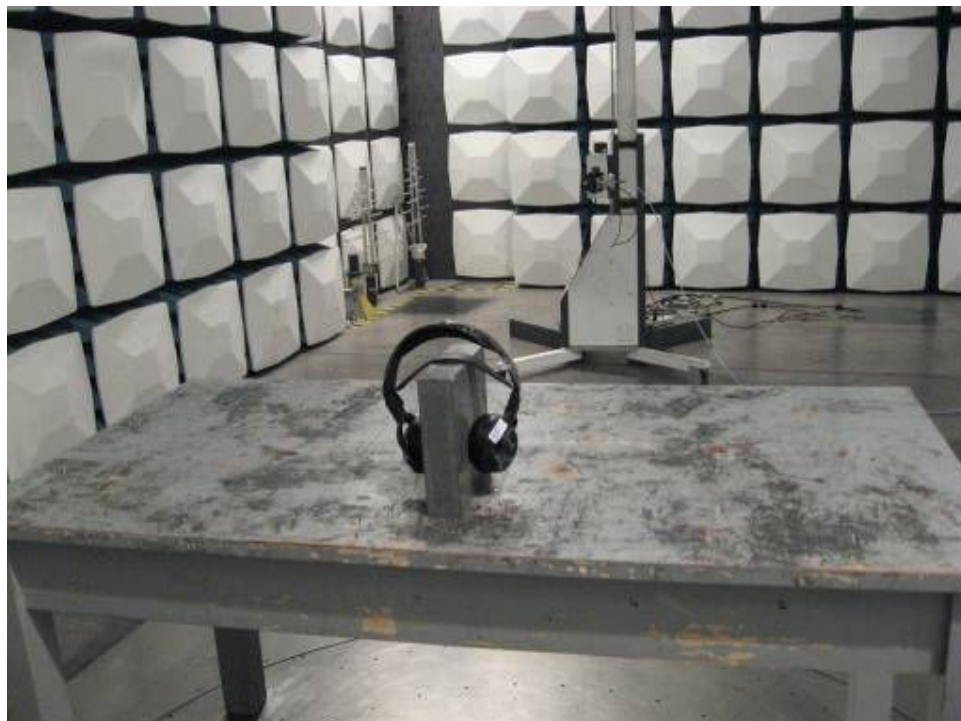
Photograph 4: Set-up for Receiver Spurious Emissions 18GHz – 26.5GHz
