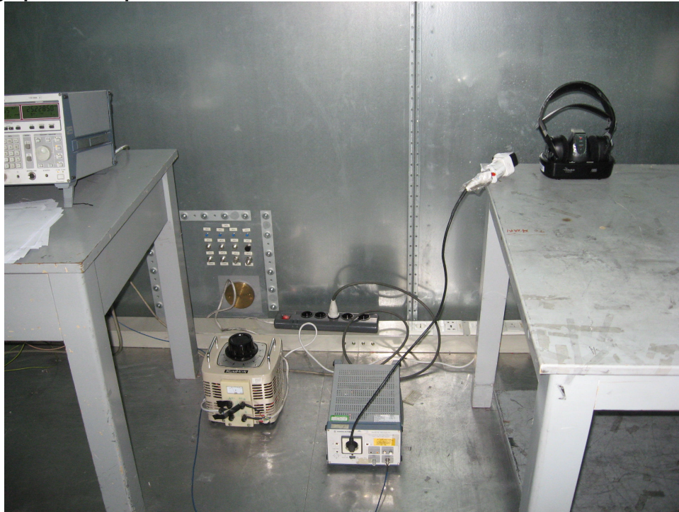
Photograph 5: Set-up for Conducted Emissions
