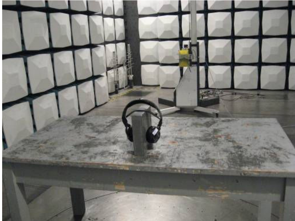
Photograph 4: Set-up for Receiver Spurious Emissions 18GHz – 26.5GHz
