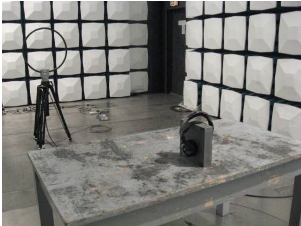
Photograph 2: Set-up for Receiver Spurious Emissions 30MHz – 1GHz
