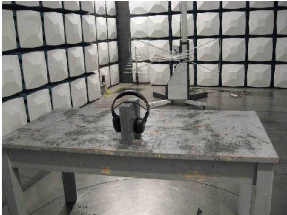
Photograph 2: Set-up for Receiver Spurious Emissions 30MHz – 1GHz
