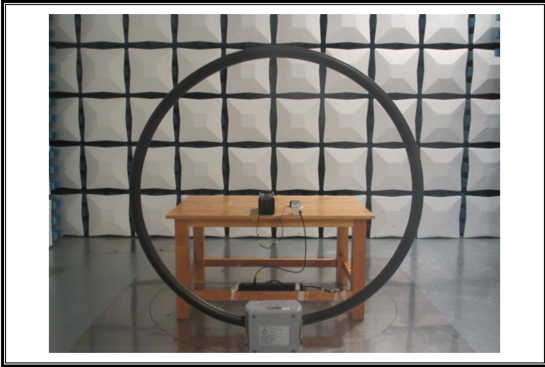
RADIATED RF MEASUREMENT SETUP (30MHz ~ 1 GHz)
