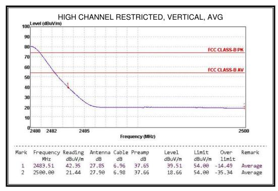
Note: EUT in each of three orthogonal axis emissions had been tested, but only the worst case (X axis) data recorded in the report.
