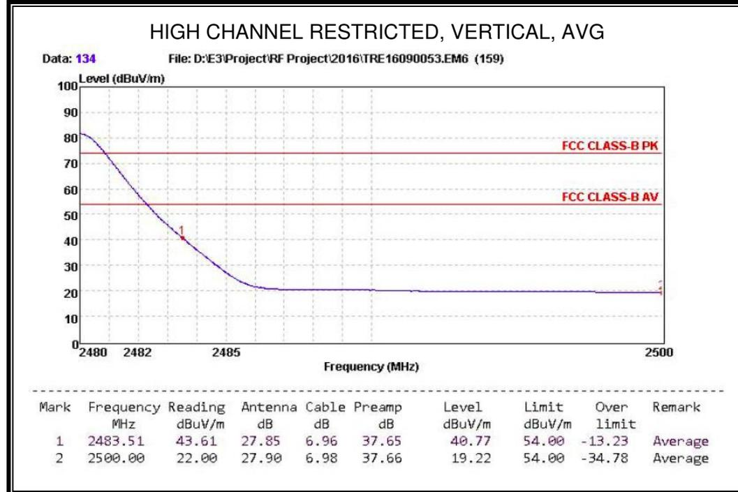
Note: EUT in each of three orthogonal axis emissions had been tested, but only the worst case (X axis) data recorded in the report.
