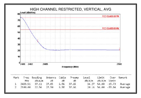
Note: EUT in each of three orthogonal axis emissions had been tested, but only the worst case (Z axis) data recorded in the report.
