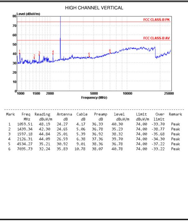
Note: EUT in each of three orthogonal axis emissions had been tested, but only the worst case(Z axis) data recorded in the report.
