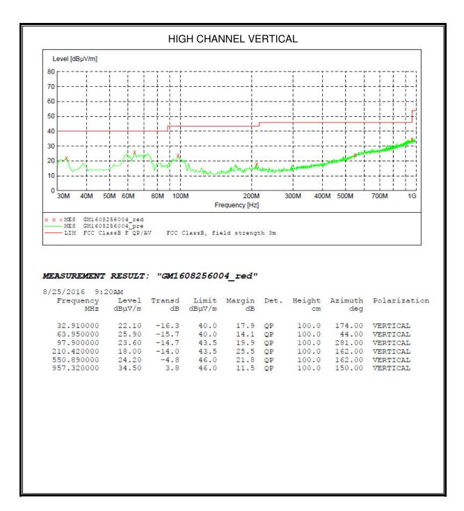
Note: EUT in each of three orthogonal axis emissions had been tested, but only the worst case (X axis) data recorded in the report.
