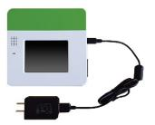
Kinoma Create uses special charging circuitry and requires a sensing charger to correctly charge the battery. Only use the provided charger, since other chargers may not charge the battery
