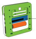
**Rear Pins:** The 50 pins accessible behind the rear access panel have dedicated functionality to support Digital, Analog Input, PWM, I2C, and Serial connections. Power can be supplied at 3.3 or 5 volts. Input pins will handle up to 3.3v.
