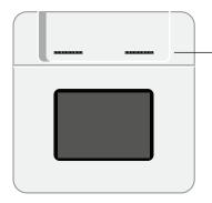
**Front Pins:** The 16 front facing pins can be targeted by the Front Pins app to support Digital, Analog In, and I2C connections. Power can be supplied at 3.3 or 5 volts. Input pins will handle up to 3.3v. The front pins are designed to conveniently fit readily-available sensors.
