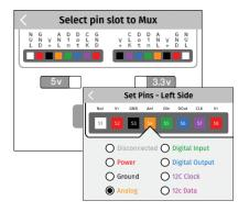
**Front Pins:** The 16 front facing pins can be targeted by the Front Pins app to support Digital, Analog In, and I2C connections. Power can be supplied at 3.3 or 5 volts. Input pins will handle up to 3.3v.
