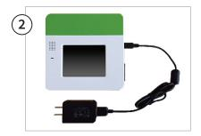
Begin charging device with supplied charger. (Note: Kinoma Create uses special charging circuitry and requires a sensing charger to correctly charge the battery. Only use the provided charger, since other chargers may not charge the battery).
