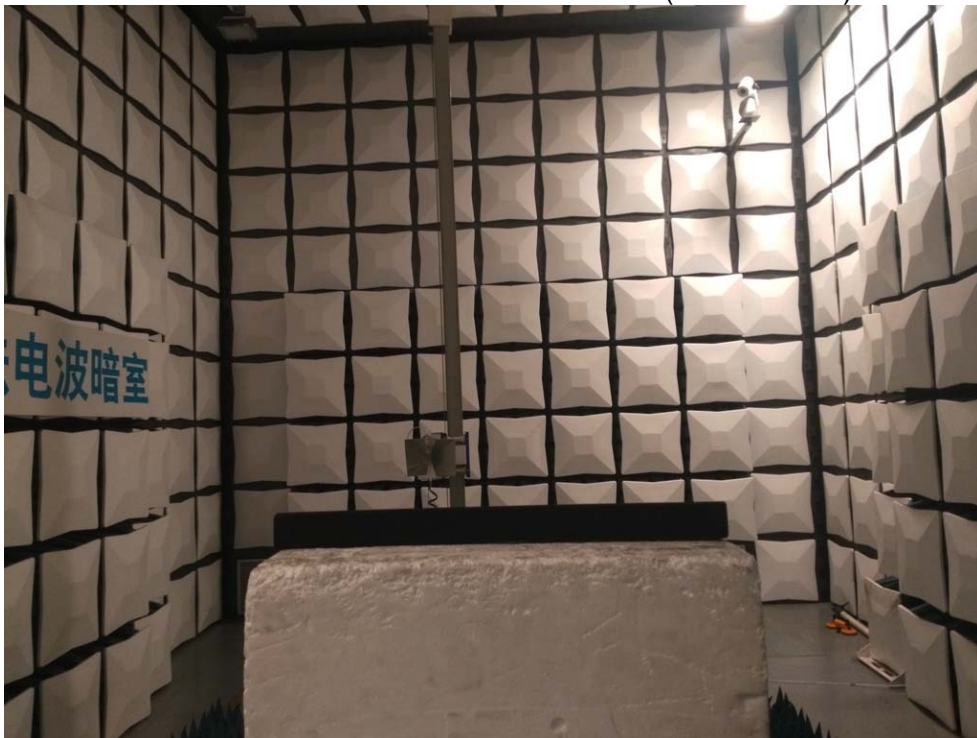
RADIATED RF MEASUREMENT SETUP (Above 1 GHz)
