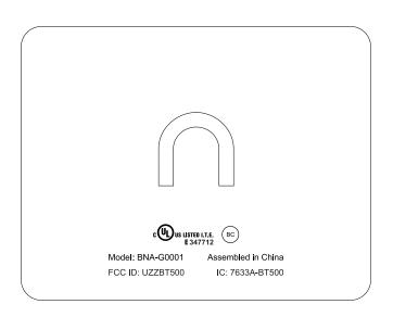
Name: Rumba BT Speaker Model #: BNA-G0001 Process: Debossed into silicone foot Finish: High Polished SPI A-2
