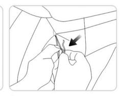
2 Black clamp connects to any iron part of car. Use the red pen to test every power line from the reverse light 3 Connect the monitor power extending line (C) to the until the LED light is on. Then you can ensure that this is the power line.
