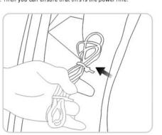
7 Connect the camera power line to the reverse light power line, anode to anode, cathode to cathode, then fix the cables with the rubberized fabric
