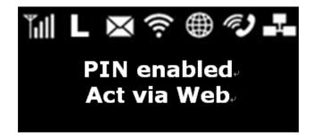
If the user has enabled the PIN security protection on the SIM card, the screen directs the user to access **4G LTE > PIN Verification** via the web interface before proceeding to use the Internet connectivity features of the device.
