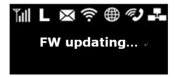
If the firmware version on the device is being updated via the Web interface, the screen informs the user of the process.
