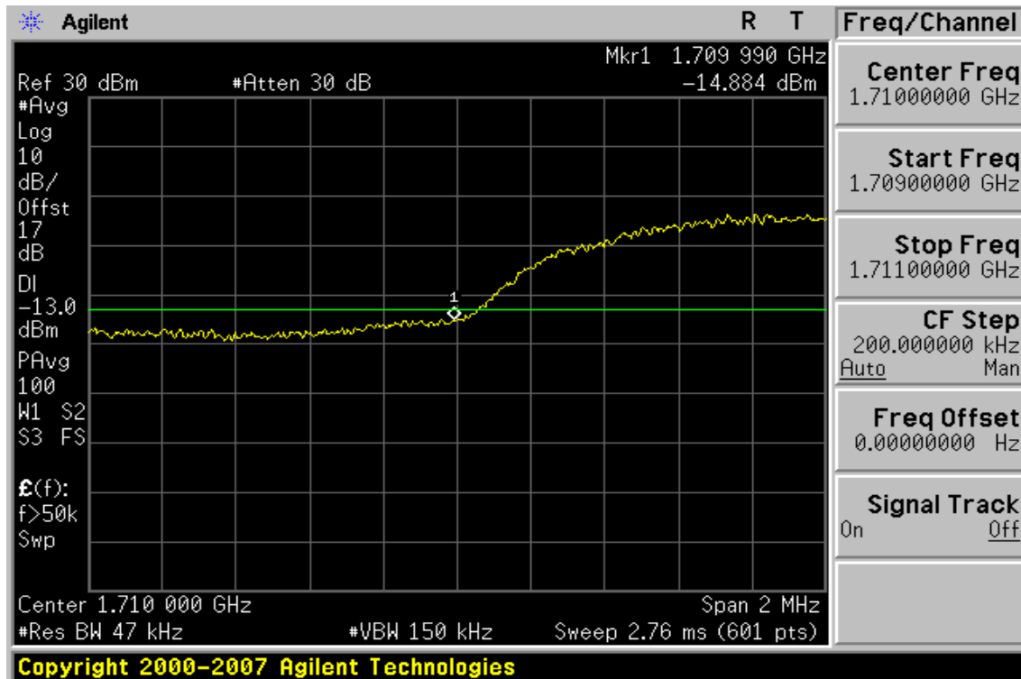
Figure 8-4: Bad edge emission at antenna terminals –WCDMA IV Channel Lowest
