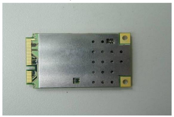
Internal of EUT - 9(WLAN module)
