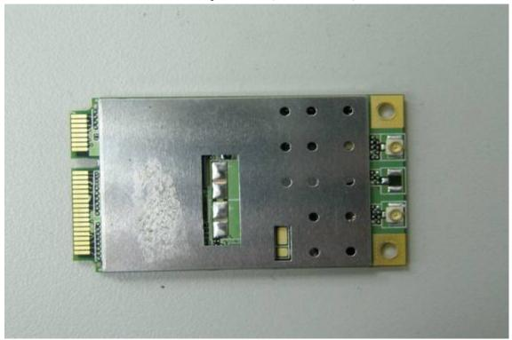
Internal of EUT – 7(GSM module)
