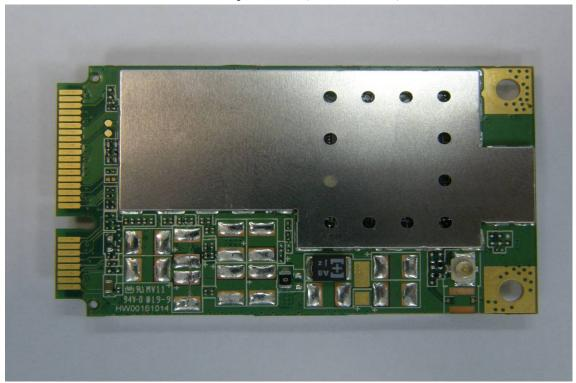
Internal of EUT – 9(GSM module)
