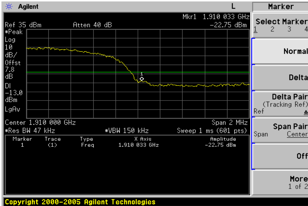
Figure 8-15: Band edge emission at antenna terminals –WCDMA II Channel Highest
