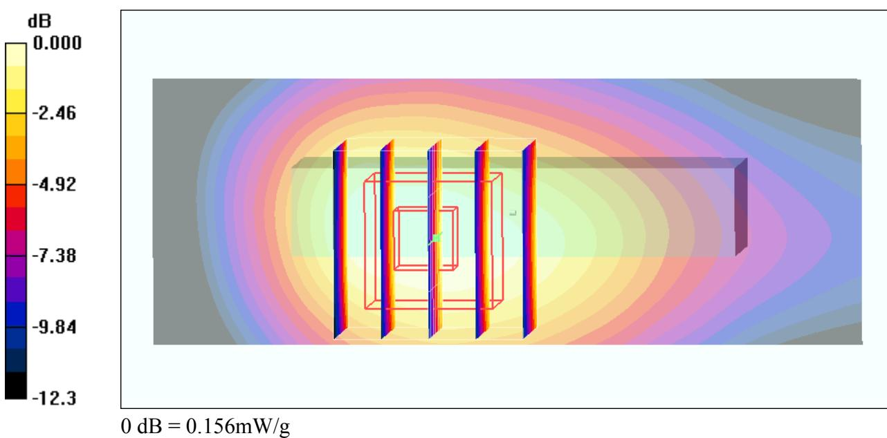
**#03 GSM850\_GPRS10\_Horizontal Down\_0.5cm\_CH189****DUT: 982031**
