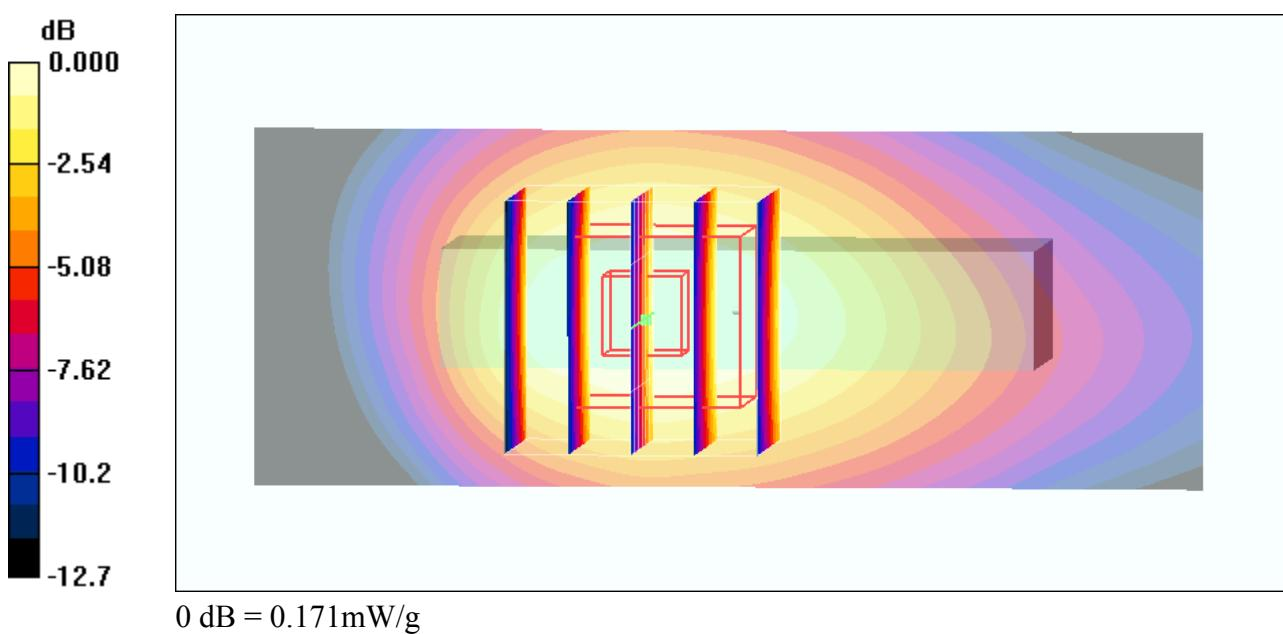
**#17 GSM1900\_GPRS10\_Horizontal Up\_0.5cm\_CH661****DUT: 982031**
