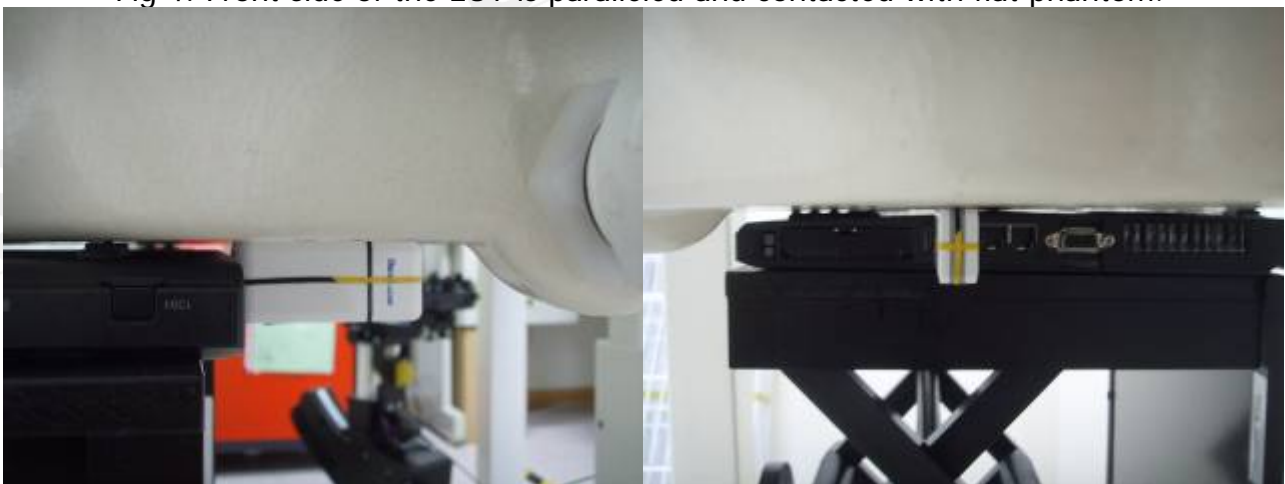
Fig 5 : Bottom side of the Notebook is paralleled and contacted with flat phantom, and left side of the EUT is paralleled with flat phantom.
