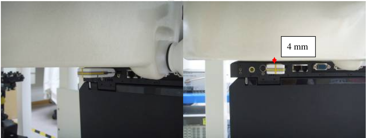
Fig 3 : Bottom side of the Notebook is paralleled and contacted with flat phantom, and back side of the EUT is paralleled with flat phantom.
