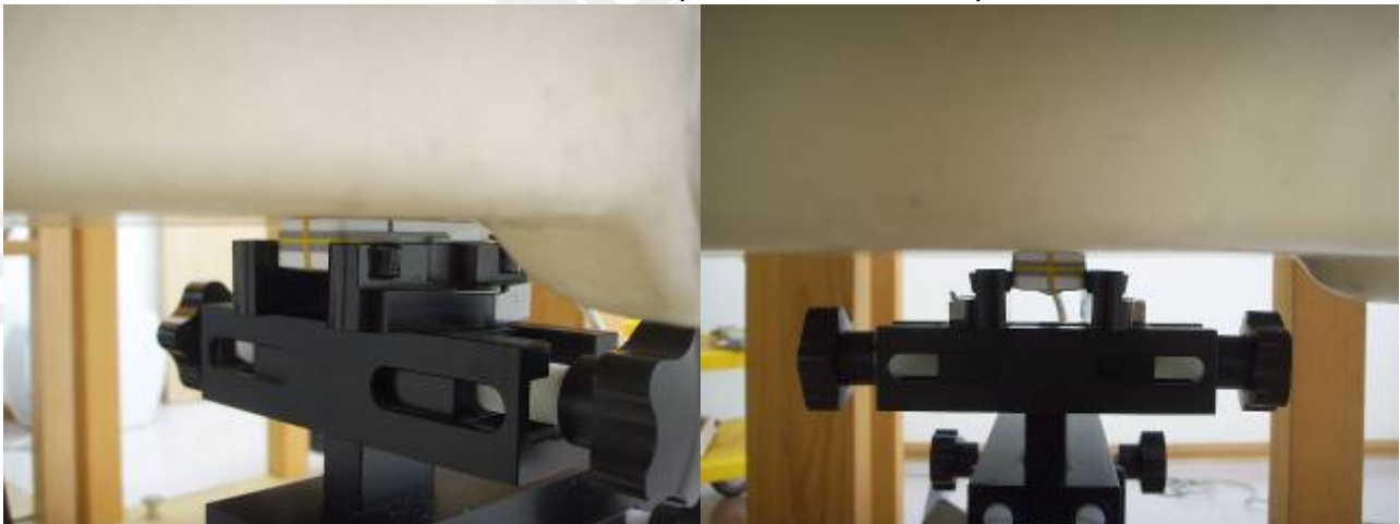
Fig 4: Front side of the EUT is paralleled and contacted with flat phantom.
