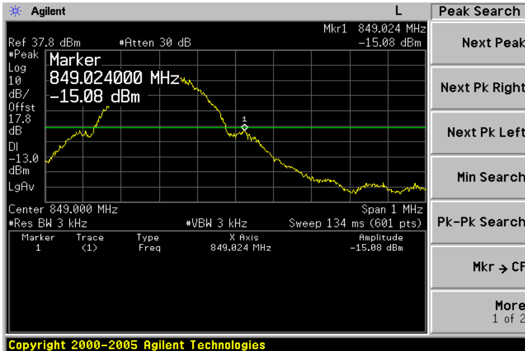
Figure 8-5: Band edge emission at antenna terminals –GPRS 850 Channel Highest
